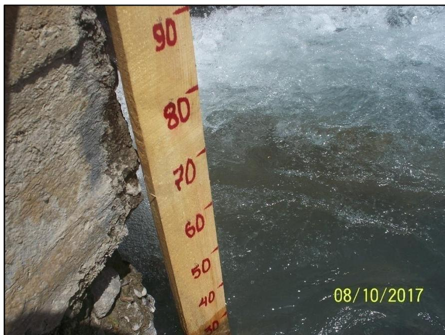
Fig. 2.12. Stake for measuring the water level in the Khodorzhiodara River on the stream gauge, on the bridge.
