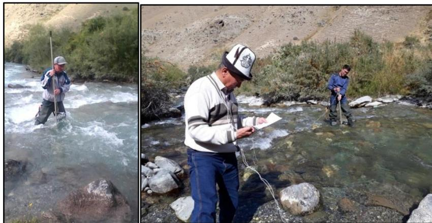
Fig. 2.1 Measurement of the depth and flow rate at the main gauging station on the Bash-Kaindy River on August 17 (left) and September 20 (right).
