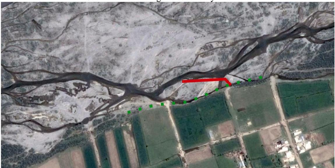
Fig.2.2.4. A fragment of the space image of 2016, showing the channel passing under the riverbank slope. The red line is a project dam about 100 m long. The green dotted line is a bush planting area.
