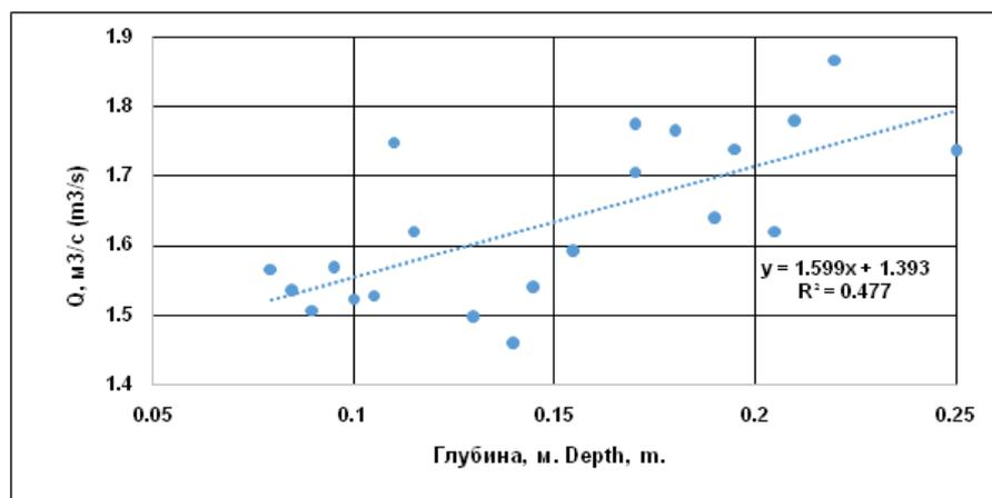
Fig. 2.18. Dependence of water discharge of the Khodorzhiodara River and corresponding change in the river's depth.
