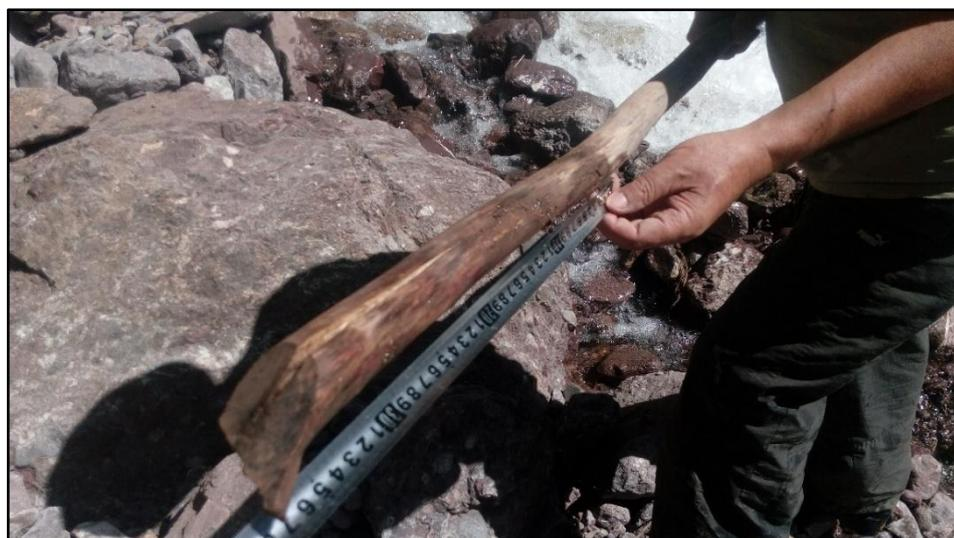
Fig.2.5. Determination of the depth of the Darzhomdara River.
