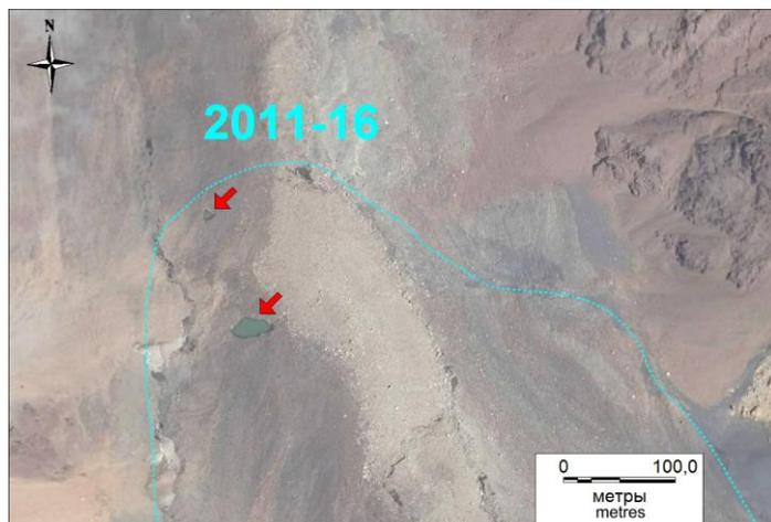
Fig. 2.5 The assumed boundary of the ice spreading under moraine cover for the period 2011-2016. Red arrows point to thermokarst funnels. Background - "WorldView 2" image from 12/08/2011.
