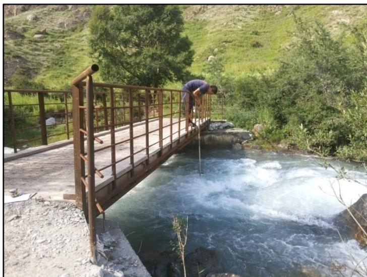
Fig.2.2 Measurement of the depth and flow velocity in July, upstream from the main gauging station, from the bridge on the Bash-Kaindy River.
