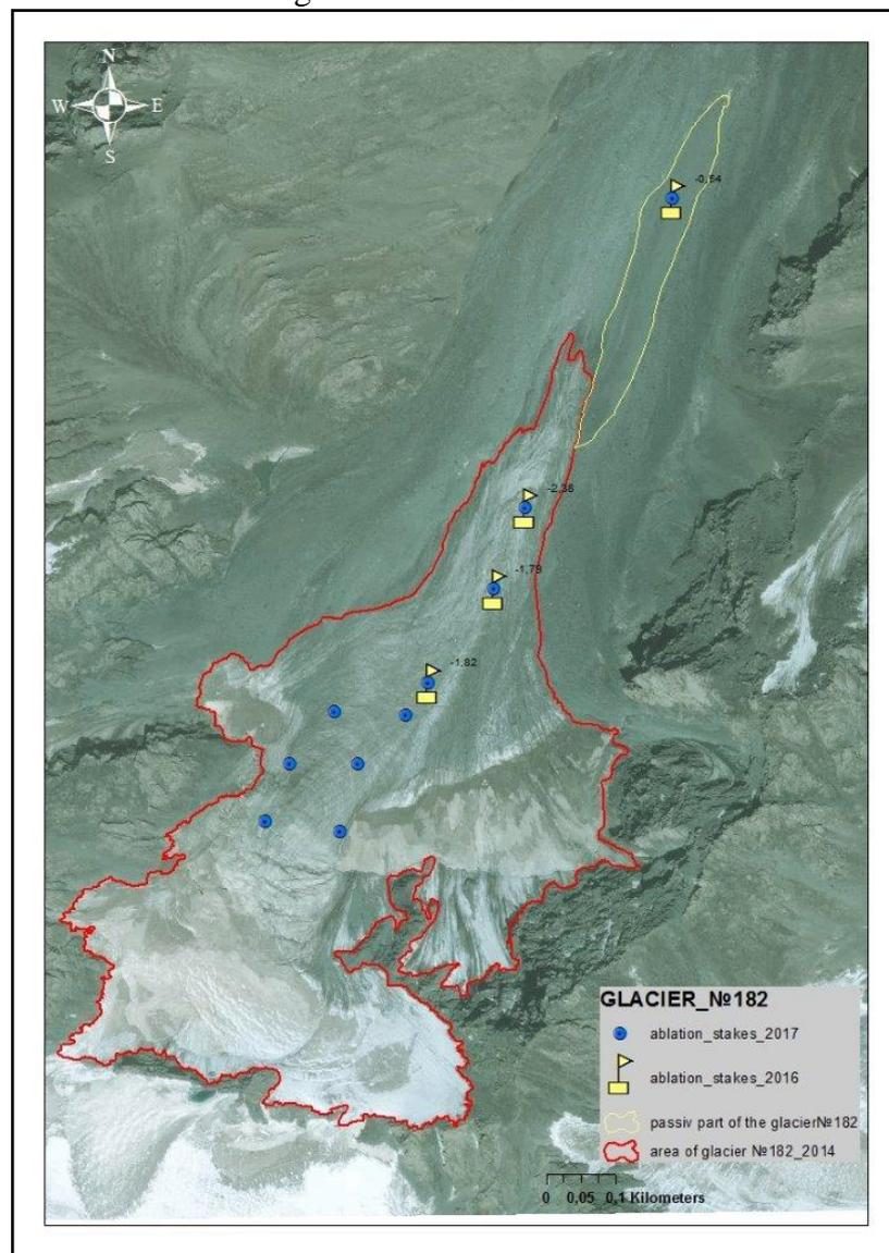
Fig.4.2 The No.182 Glacier on the "GeoEye-1" satellite image from August 1, 2014. The red line is the boundary of the glacier, the yellow line is the boundary of the passive part of the glacier separated from the active tongue of the glacier. The points are ablation rods installed in 2016 and 2017. Numbers are the ablation value in meters for the period 2016-2017.
