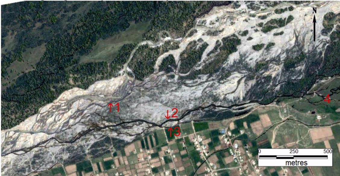
Fig.2.2.3 The "Pleiades" satellite image from May 21, 2016. 1-main riverbed of the At-Bashi River, 2 - secondary channel, 3-channel, approaching directly to the bank, 4- sources of "Kara-Suu" creeks feeding the secondary channel.
